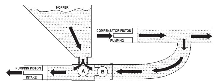
Figure 10. Pumping Cylinder
